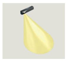
Radar sensor for detection of recognition of movement in unauthorised direction and door opening.
