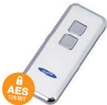
Handsender Mini-Novotron 522 Design 2-Kanal, 433 MHz, KeeLoq-Wechselcode
