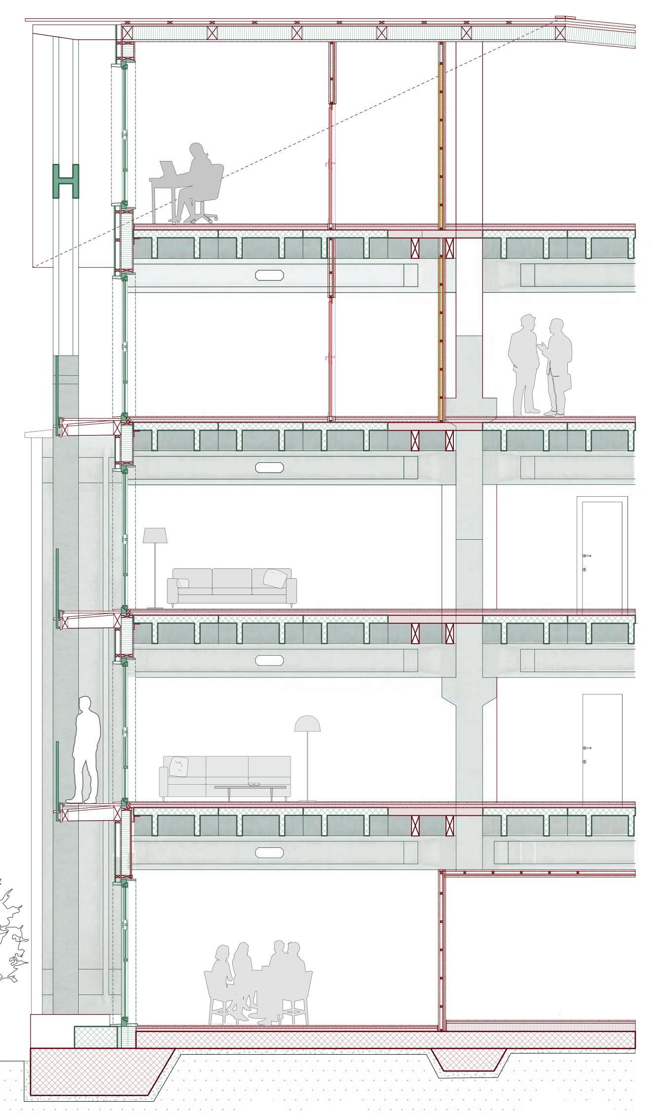
ventilation layer roofing underlay 200x60mm wood stud frame with reused mineral wool 180mm OSB boards (tongue and groove) 25mm
