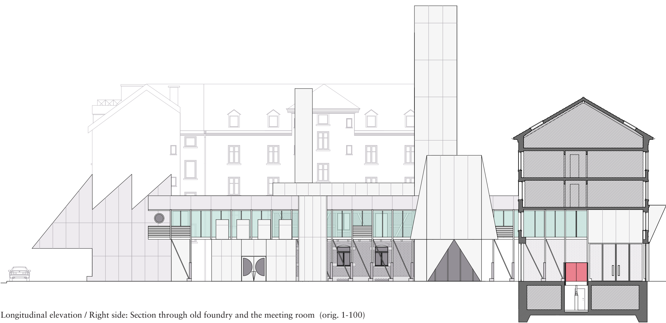
Longitudinal elevation / Right side: Section through old foundry and the meeting room (orig. 1-100)
