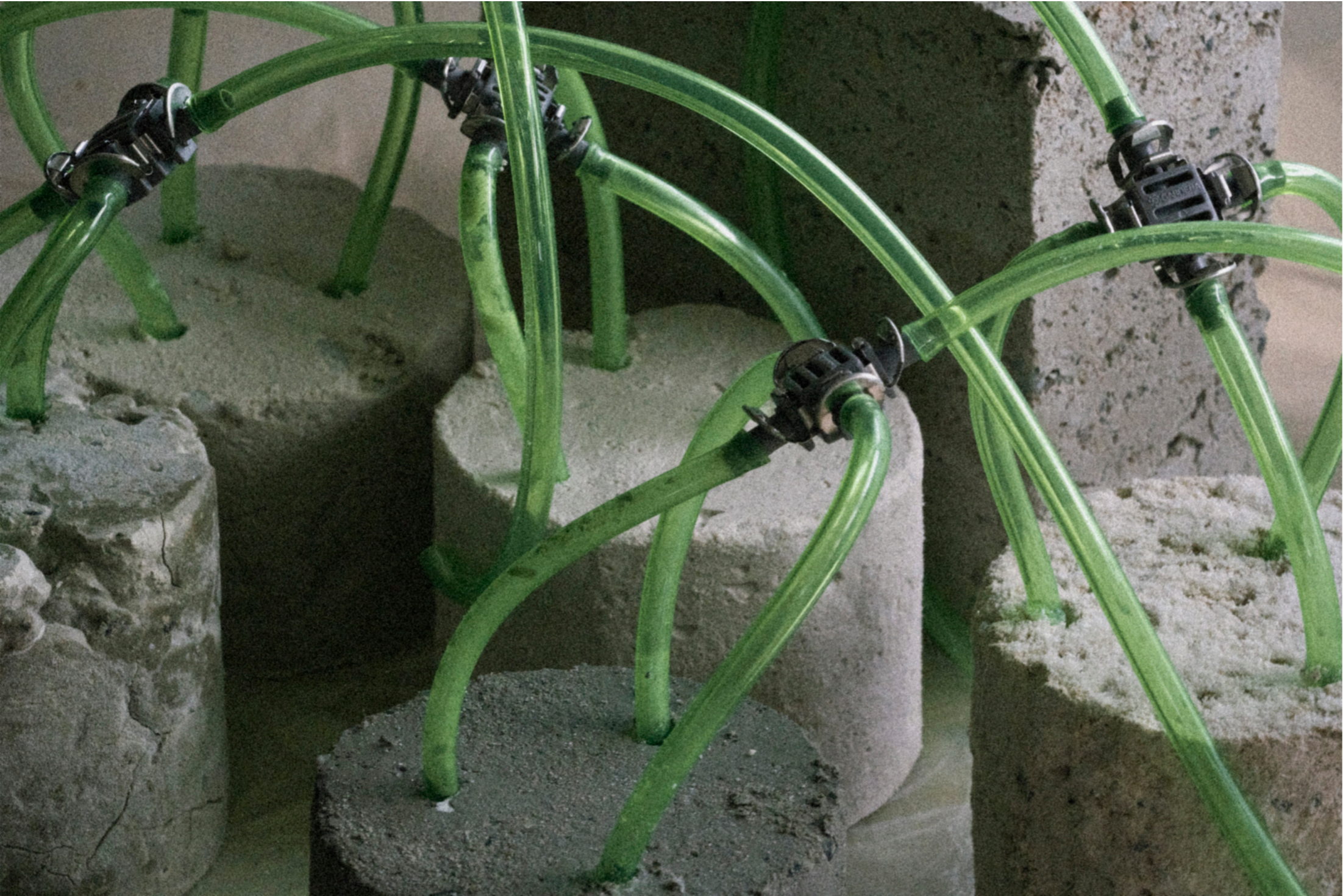
Binding material test with different mineral and natural binder
