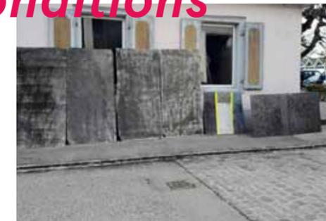
Various models made to test facade cladding are exposed to weather conditions outdoors.
